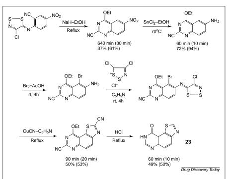
**Figure 9.** Microwave assisted synthesis of a thiazol[5,4-f]quinazoline. Numbers in brackets refer to the yields and reaction times obtained under microwave irradiation compared with conventional heating.
